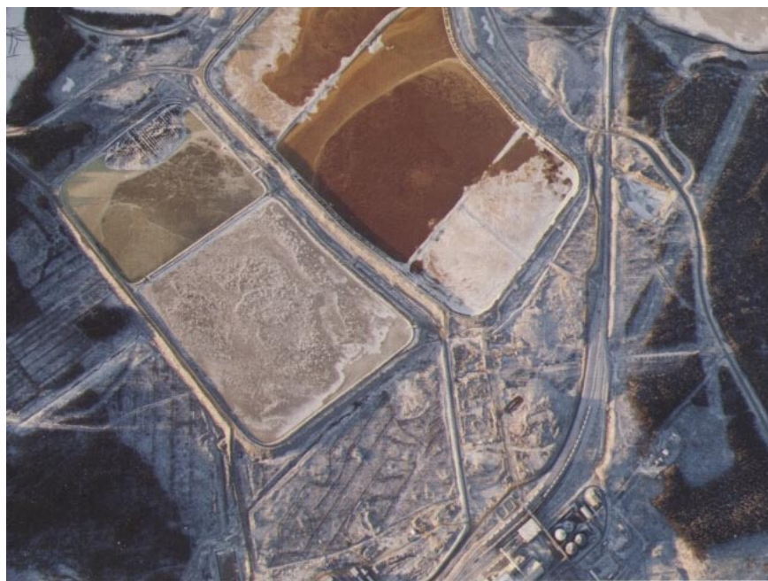
These settling ponds at the Talvivaara nickel mine in northeastern Finland accidentally discharged some two million tons of toxic mine tailings into nearby wetlands and river courses. These liquid wastes contained 6-8 tons of nickel, 1,000 kilos of uranium and 400 tons of aluminum and other heavy metals. Moreover, seepage from these ponds can contaminate groundwater, poisoning water supplies for dozens of communities.
